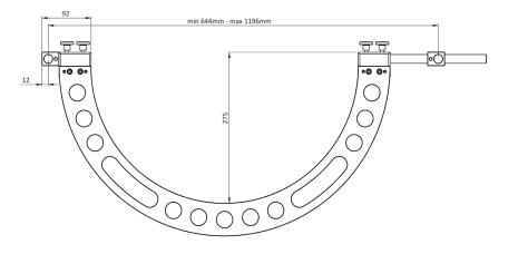
Arc configuration with blocks mounted outwards.
