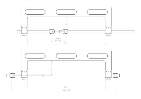
Arc configuration with blocks mounted outwards.
